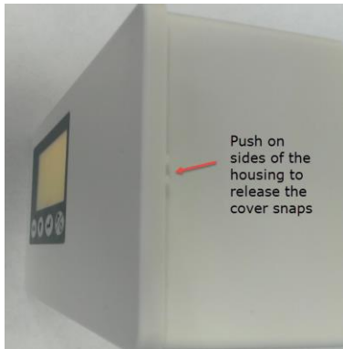
Fig. 1-3 Removing bezel from the base
